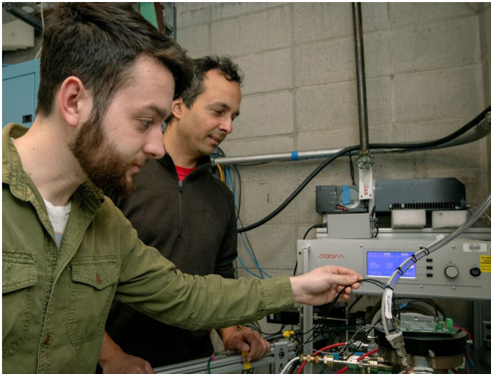
Figure 2. Will Larsen and Arun Persaud at the neutron test facility of the Fusion Science and Ion Beam Technology Program in the Accelerator Technology & Applied Physics Division, configuring the alpha particle detector. The alpha detector allows the measurement of the distribution of carbon atoms in soil. Credit: Berkeley Lab
